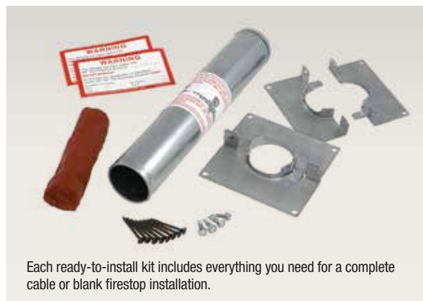
Label holds sleeve together until you need to retrofit around existing cables. Slit label to open sleeve. Close the two halves around the cables.
