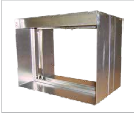
FDD-SB Curtain Fire Damper - 1-1/2 & 3 Hour - Dynamic or Static - Integral Sleeve, Type B
