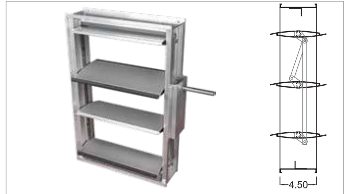
CD-150 Opposed blade control, extruded aluminium airfoil blades, up to 13" w.g
