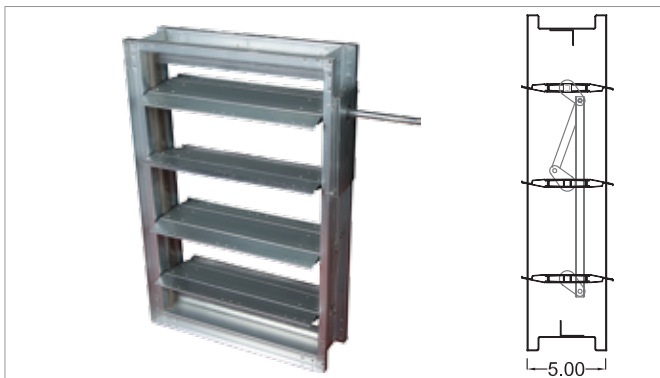
CD-160 Opposed blade control, airfoil blade steel, up to 13" w.g (Roll-formed)
